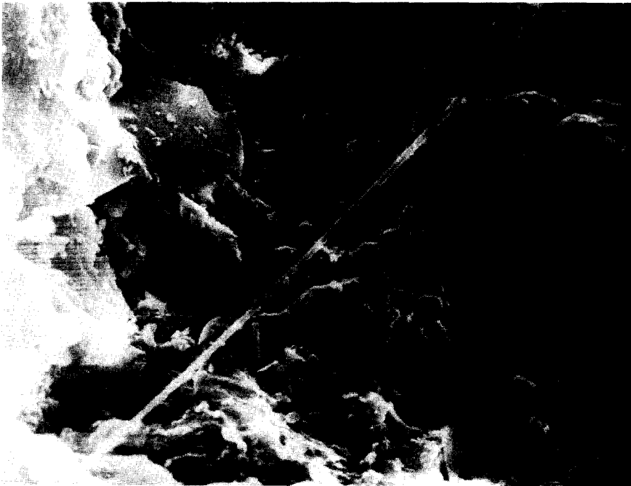
FIG. 10. The 9% Ni, 1.5% Pt catalyst exposed to CO at 300°C.
