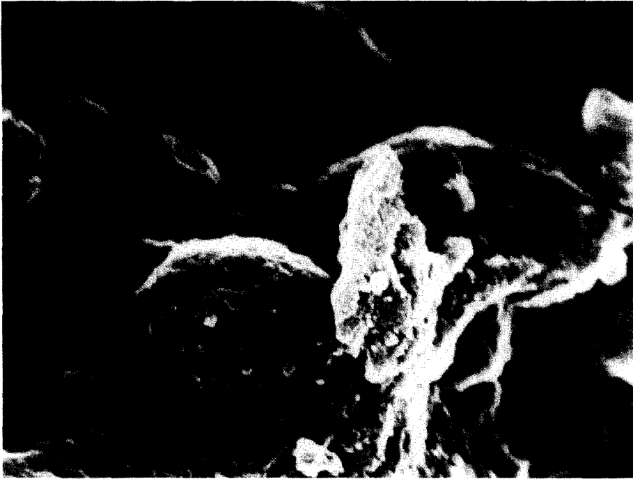
FIG. 9. The 9% Ni catalyst totally deactivated by a methanation reaction.
